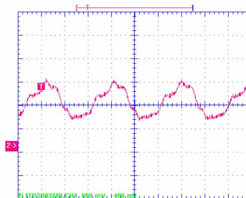
Figure 8: Friction curve at 15 N loading
