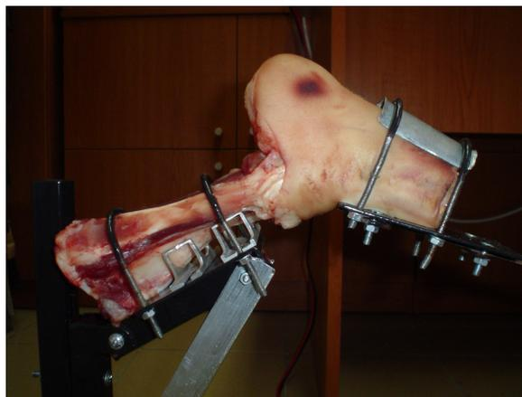
Figure 4: Joint clamped on the experimental apparatus
